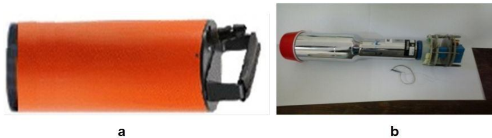
Figure 7. Gamma-sensor probe, GSP-3 (a), scintillation crystal optically tight to a photomultiplier in a scintiblock and electronic circuit (b).
