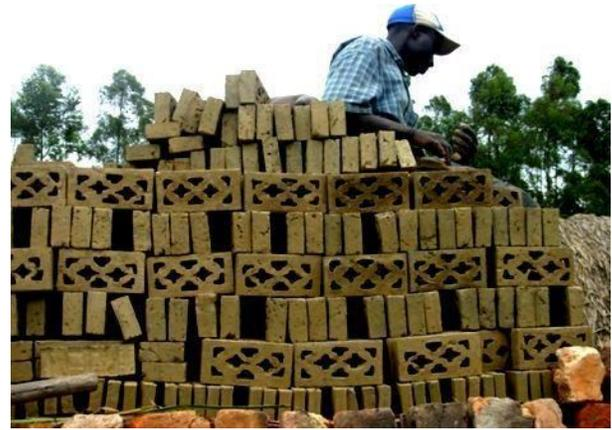
**Figure 18.** Stacking ventilators on a field kiln.
