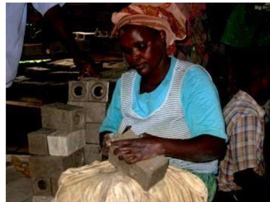
**Figure 16.** Trimming bottom brick plates.
