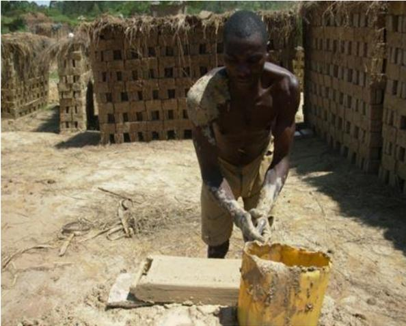
**Figure 7.** Brick making using a wooden mould.
