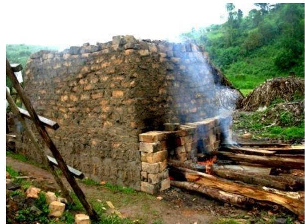
**Figure 19.** Firing ventilators in a field kiln.
