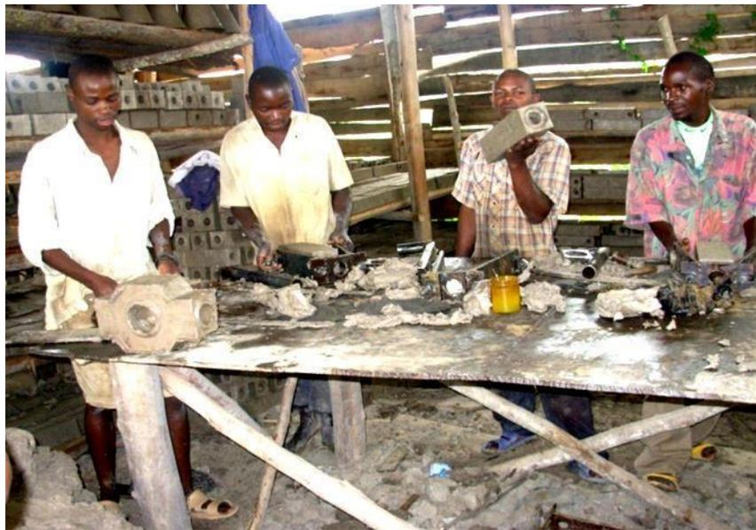
**Figure 14.** Forming process of bottom brick plates.
