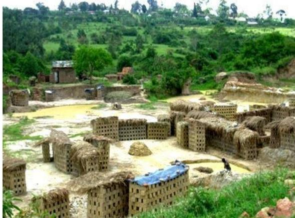
**Figure 8.** Stack bricks covered with grass.
